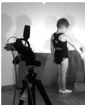
**Figure 1.** Arrangement of the retroreflective markers on the body of the subject
